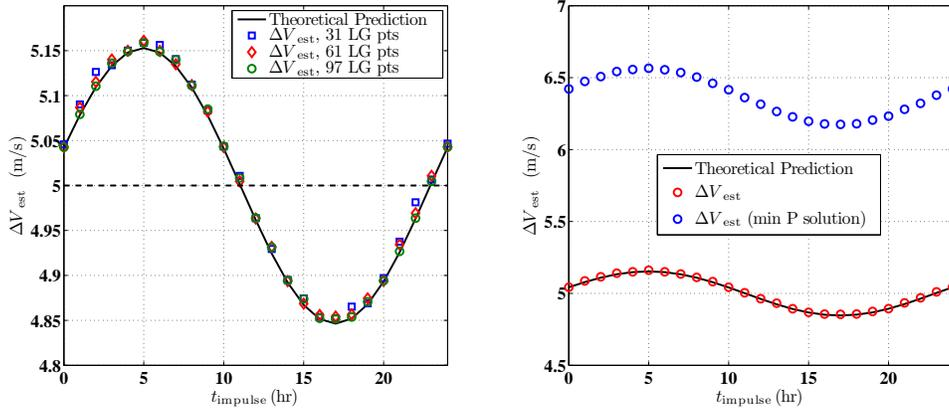
**Figure 6.** Comparison of  $\Delta V$  (estimates vs. theoretical prediction) obtained for inclination-only maneuvers (left), and comparison with estimates obtained from minimum “energy” solution (right). The sinusoidal shape is due to the fact that the change in inclination  $\Delta i$  itself oscillates as a function of the impulse time due to the gravity model.
