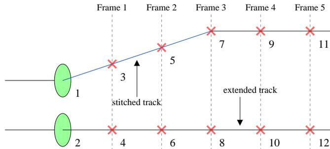
**Figure 3. The result of applying a post-processor track stitching algorithm to connect disparate tracks, UCTs, and false alarms by way of an optimal control.**
