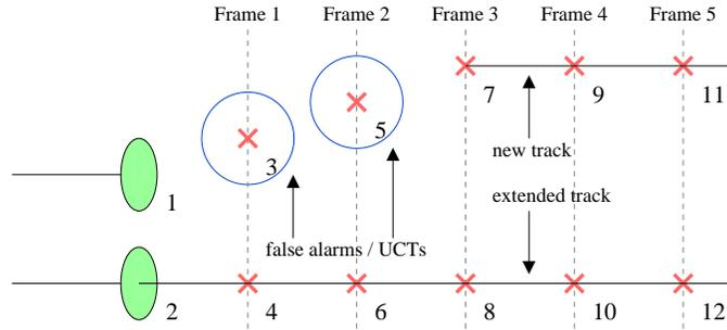
**Figure 2. Tracks, UCTs, and false alarms generated by running an MHT without maneuver detection.**
