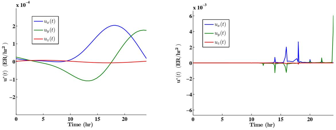
**Figure 4. The optimal control profile obtained for Scenario  $3_{sb}$ . Shown are the minimum energy solution (left) and the minimum  $\Delta V$  solution (right).**
