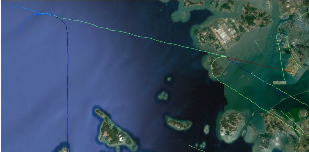
Figure 18. Here the attribute estimate ambiguity resulting from the ambiguous data association regions is shown, with most of the tracks having no attribute information, two having an initial (dark) blue attribute and one having a red attribute.
